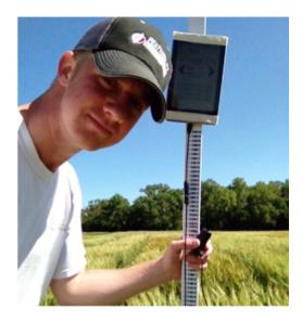
Fig. 1: Plant height measurement via barcoded height stick
